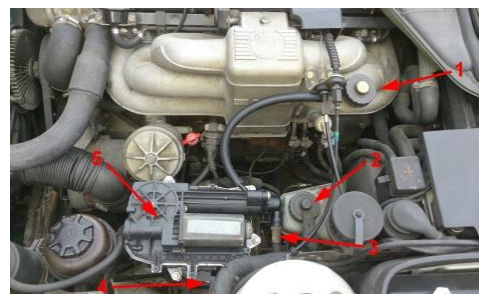
Fig. 3. Installation of electrohydraulic clutch cylinder and main control unit: 1-Liquid container for automatic clutch, 2- Liquid container for manual clutch, 3- Connecting the electrohydraulic cylinder to the original clutch system, 4- Connecting the wiring to communicate with the car, 5- Electrohydraulically coupled cylinder
