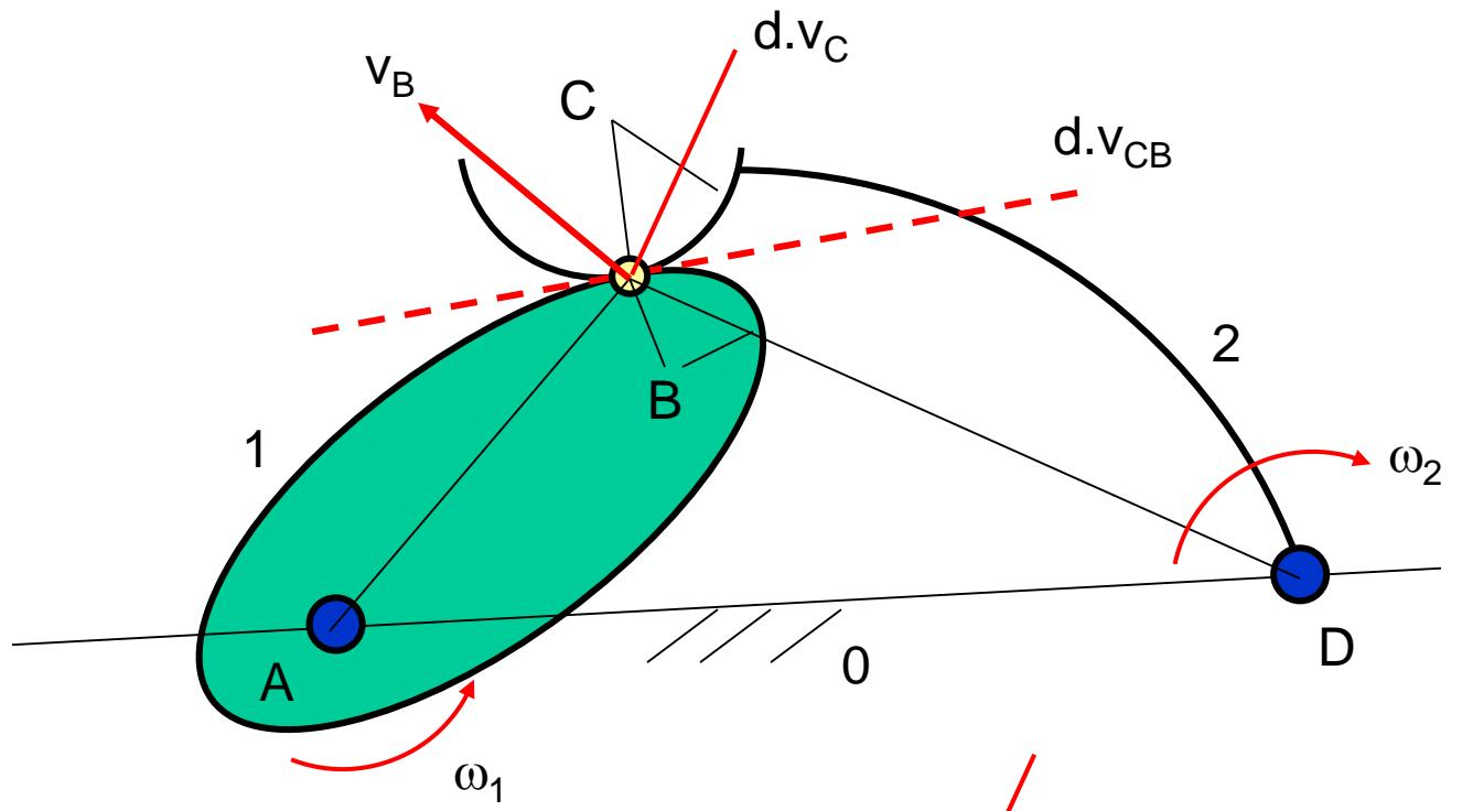
$$\underline{\underline{v}_C} = \underline{\underline{v}_B} + \underline{\underline{v}_{CB}}$$
