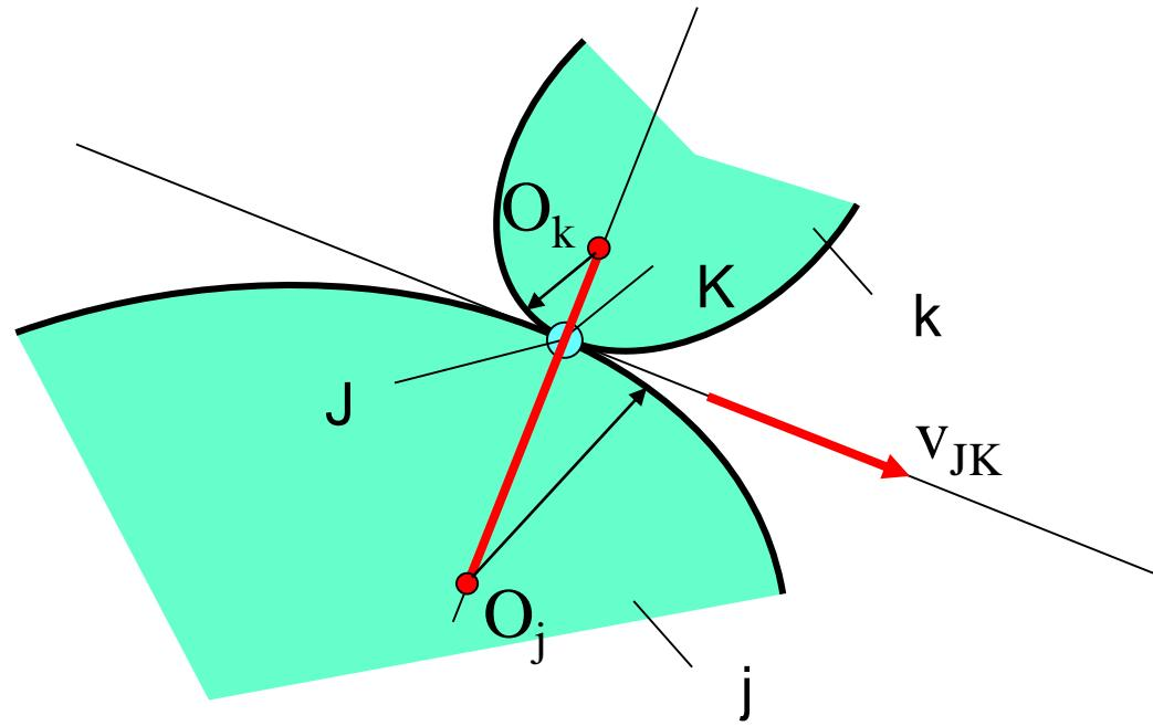
$$\text{Velocity: } v_J = v_K + v_{JK}$$
