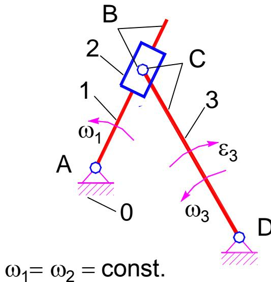
$$\underline{\underline{\mathbf{a}_C^n}} + \underline{\underline{\mathbf{a}_C^t}} = \underline{\underline{\mathbf{a}_B^n}} + \underline{\underline{\mathbf{a}_{CB}^C}} + \underline{\underline{\mathbf{a}_{CB}^t}}$$
