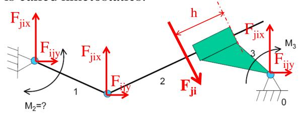
Number of equations = numer of uknown variables Number of equations = (numer of moveable links)  $x = 3 \times 3 = 9$ numer of uknown variables = (uknown balancing moment) + (unknown components of forces in kinematic pairs) =
